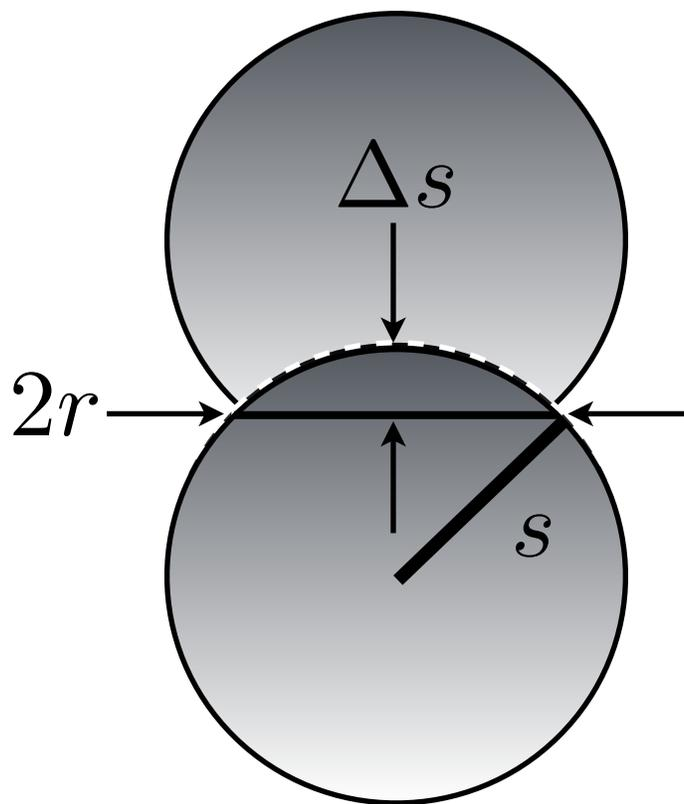
Figure 1: Two smooshed spheres. Notwithstanding the author's ineptitude with Keynote, both spheres are smooshed inward by  $\Delta s$ . The radius of the smooshed, flattened cap is  $r$ .
