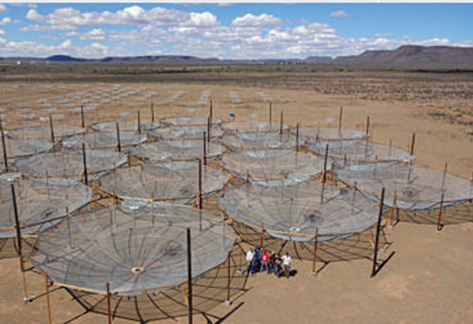
The HERA array in South Africa consisted of 19 dishes on March 7, 2016, but continues to grow, replacing an earlier experiment called PAPER (small dishes in the background). (Images courtesy of the HERA team)
