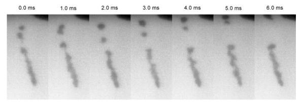
Fig. 7. Comet-like streamers (C<sub>3</sub>H<sub>6</sub>O, 4 °C,  $\sim \pm 17$  bars, 16.0 kPa).
