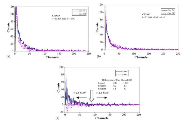
Fig. 5. (a) Representative neutron gated counts below and above 2.5 MeV proton recoil edge for tests with  $C_3D_6O$  at  $\sim$ 0 °C with and without cavitation; (b) representative neutron gated counts below and above 2.5 MeV proton recoil edge for tests with  $C_3D_6O$  at  $\sim$ 0 °C with and without cavitation; (c) representative neutron gated counts below and above 2.5 MeV proton recoil edge for tests with  $C_3D_6O$  and  $C_3H_6O$  at  $\sim$ 0 °C with and without cavitation.
