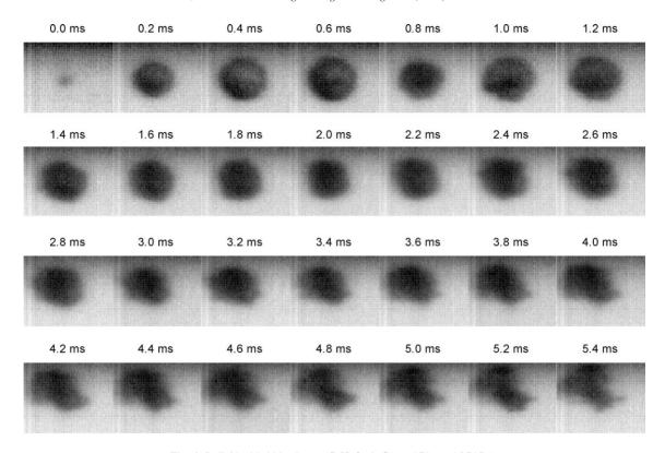
Fig. 6. Individual bubble cluster (C3H6O,  $4\,^{\circ}\text{C}$  ,  $\sim\!\pm17$  bars, 16.7 kPa).
